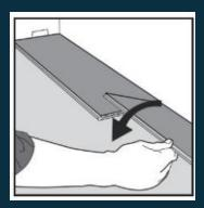
4. Press down with your hand or tap lightly with a rubber mallet on the tile you just installed.
